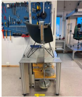
EN1022:2018 7.3.5.2 Sideways overturning
