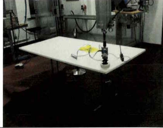
Picture. 2: Vertical static load test
