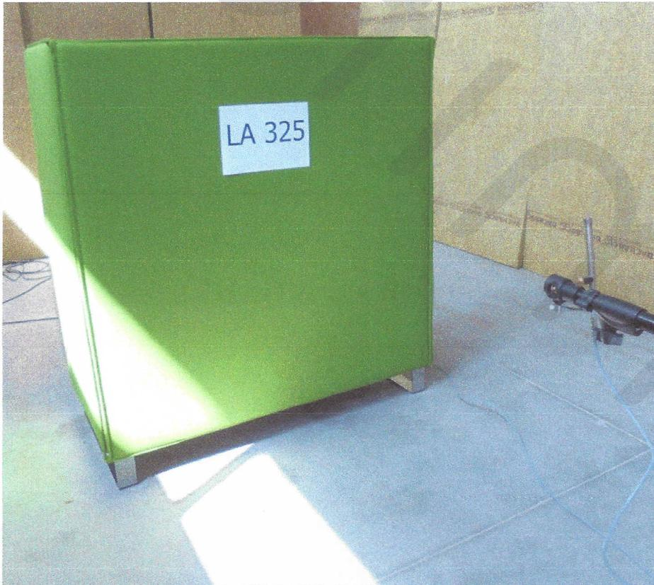
Fig. 3. Placing the microphone at a distance of 140 cm from a screen
