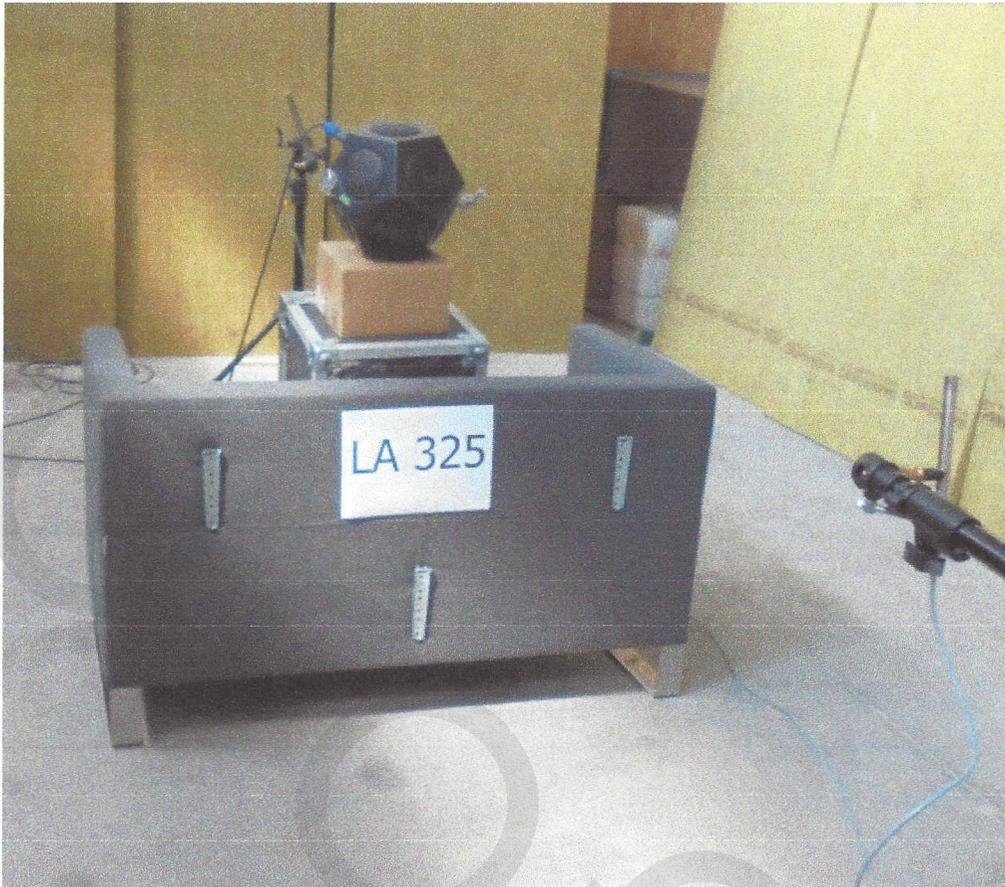
Fig. 4. Placing the microphone at a distance of 140 cm from the sofa without a screen
