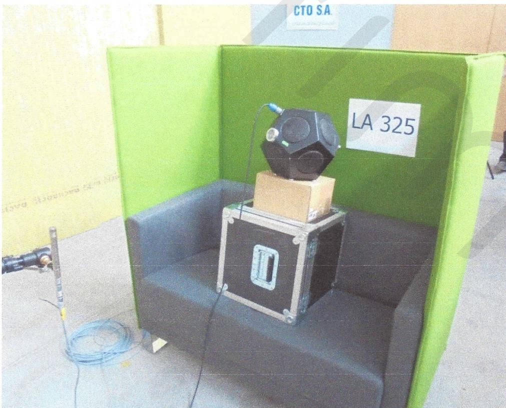
Fig. 5. Placing the sound source on the sofa at a height of 110 cm
