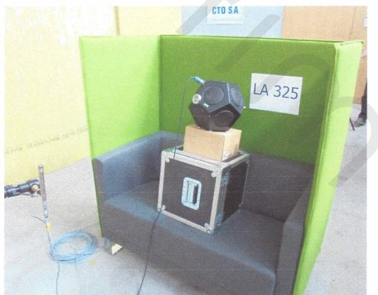
Fig. 5. Placing the sound source on the sofa at a height of 110 cm
