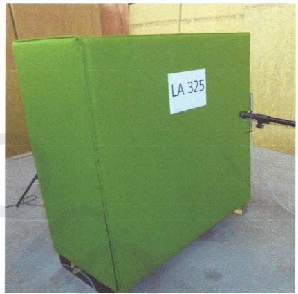
Fig. 2. Placing the microphone at a distance of 35 cm from a screen
