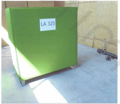
Fig. 3. Placing the microphone at a distance of 140 cm from a screen
